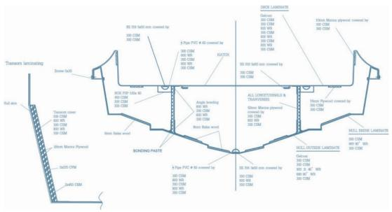
Hand lay-up laminate schedule with plywood core
